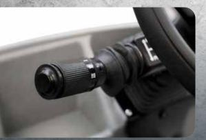
3 pre-set speeds selectable from the forward/reverse lever, allowing the floor scrubber to perfectly adapt to surfaces and specific cleaning needs in any environment.
