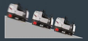
Machine slowdown on downhill slopes to allow the operator to maintain constant control and avoid sudden braking.
