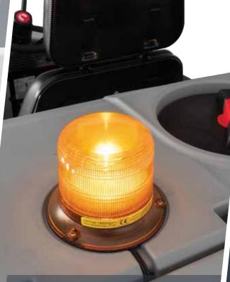
Blinking light that automatically activates when the floor scrubber is turned on, to signal that the machine is moving. The buzzer also provides an acoustic warning when C 130 moves in reverse, the warning can also be activated manually when moving forward.
