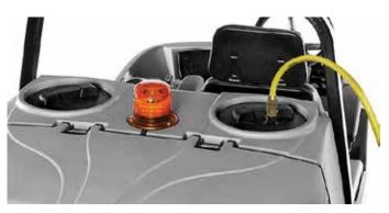
FFS – Fast Filling System, the optional technology of Comac that allows to fill the water tank with a special device, this operation does not require the presence of the operator and thus contributes to reducing the downtime of the machine.
