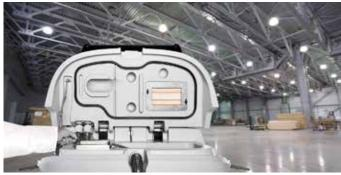
To always achieve high performance, it is essential to regularly clean the suction filter, capable of retaining dust and protecting the suction motors from foams and detergents, and the basket filter, which thanks to its conformation, it can retain debris to prevent it from settling on the bottom of the recovery tank.
