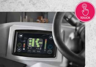
7" touchscreen display perfectly positioned to ensure good interaction with the operator while driving and easy access to all machine functions.
