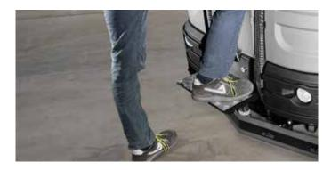
The C130 is also equipped with some small features that make it easier for the operator to carry out daily maintenance, like the convenient platform located at the back of the machine that allows the operator to easily inspect the tanks and filter systems of the scrubber.
