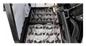
Automatic refilling of the batteries, which tanks to a single circuit, connects all the elements and allows you to adjust the level of filling from a single point. The refill is therefore much faster as it greatly reduces stops, and safer, since you avoid leakage of electrolyte from the batteries.
