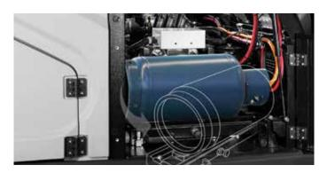
In the Bi-Fuel version, a special compartment has been made for the LPG cylinder, which can be easily removed thanks to a convenient support that rotates towards the outside of the machine.
