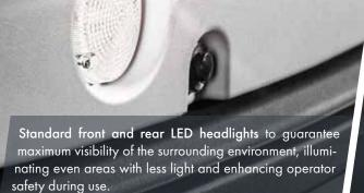
Rear headlights that include position, reverse, and stop lights to signal the machine's presence at all times.
